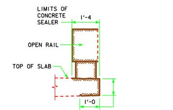
**CONCRETE SEALER LIMITS FOR OPEN RAILS**
