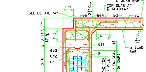
**SECTION NORMAL TO ABUTMENT AT C**
