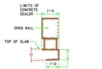
**CONCRETE SEALER LIMITS FOR OPEN RAILS**
