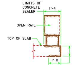
**CONCRETE SEALER LIMITS FOR OPEN RAILS**
