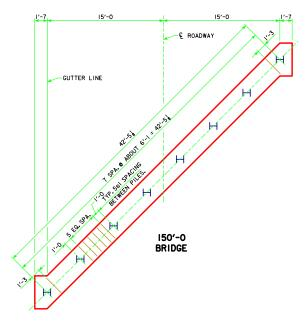
NOTE: ALL PILES ARE TO BE ORIENTED WITH WEBS PERPENDICULAR TO THE  $\widehat{\mathbb{Q}}$  OF THE ROADWAY AS SHOWN.
