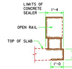
**CONCRETE SEALER LIMITS FOR OPEN RAILS**
