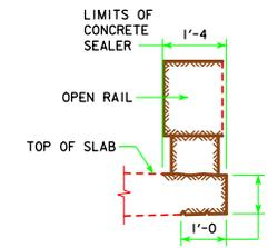
**CONCRETE SEALER LIMITS FOR OPEN RAILS**
