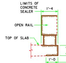
**CONCRETE SEALER LIMITS FOR OPEN RAILS**
