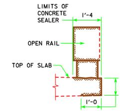
**CONCRETE SEALER LIMITS FOR OPEN RAILS**
