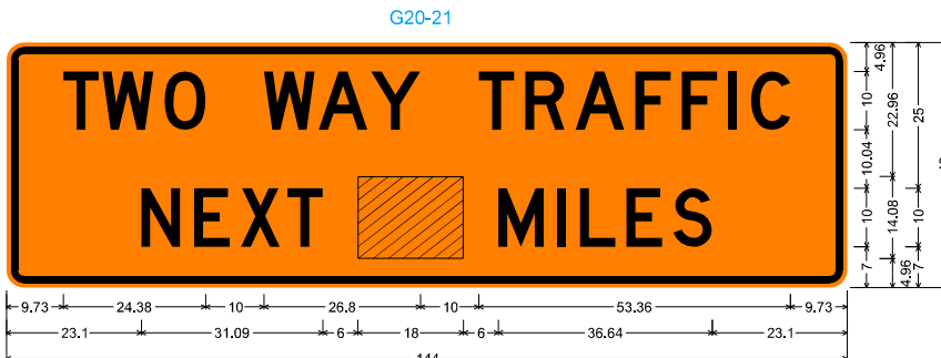
G20-21: 3.00" Radius, 1.25" Border, 0.75" Indent, Black on Orange; [TWO WAY TRAFFIC] D; [NEXT] D; Rectangle Orange; [MILES] D;
