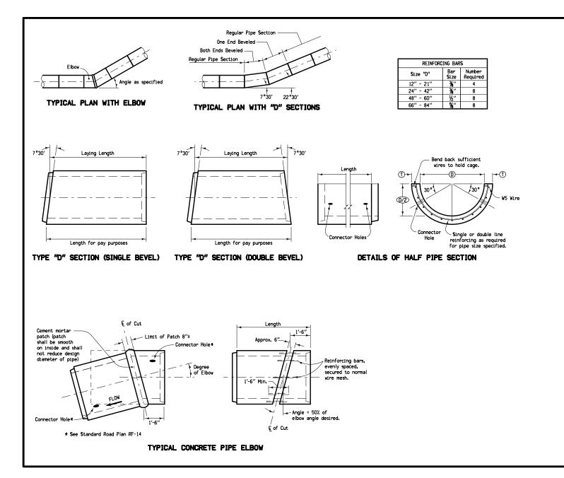
Fabricate concrete pipe elbows and Type "D" pipe sections in conformance with AASHTO M 170 for the size and class of pipe specified.
