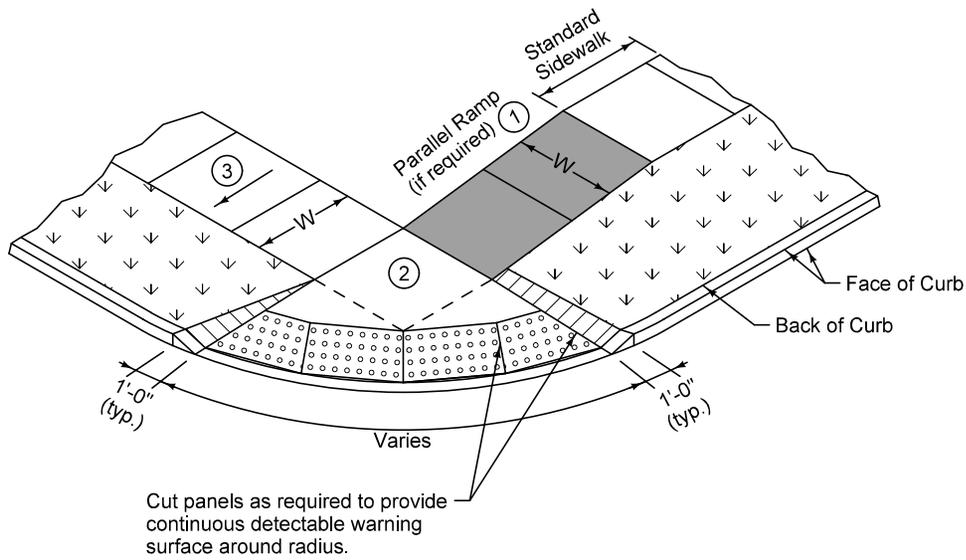
① Parallel Curb Ramp: If normal sidewalk elevation cannot be achieved with the perpendicular ramp between the street and landing due to limited ramp length, provide a parallel ramp to make up the elevation difference between the landing and the standard sidewalk.
