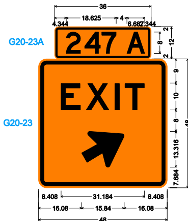
G20-23A; 1.500" Radius, 0.625" Border, 0.375" Indent, Black on Orange; [247] D; [A] D; G20-23; 3.000" Radius, 1.250" Border, 0.750" Indent, Black on Orange; [EXIT] E; Arrow K-17, 30°;
