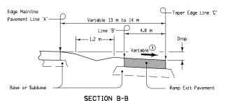
Ramp exit pavement shall be the same thickness as mainline pavement.
