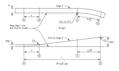
${\sf CASE\ B}$  Normal Pavement Sloped in the Same Direction as Superelevation
