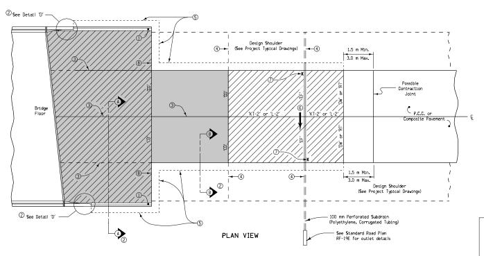
Build 100 millimeter Sloped Curb to end of Double Reinforced Section.
