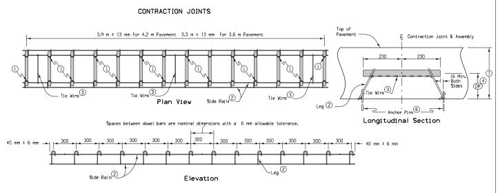
Dowel bars shall be 460 mm long with a tolerance of  $\pm$  3 mm. The centerline of individual dowels shall be parallel to the other dowels in the assembly within ± 3 mm.
