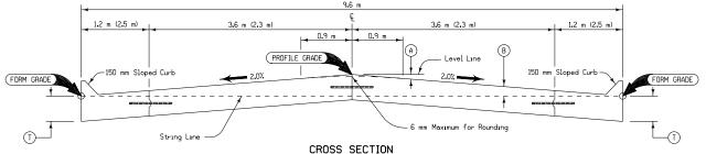
(Dimensions in (##) for  $\bigcirc$  less than 230 mm)
