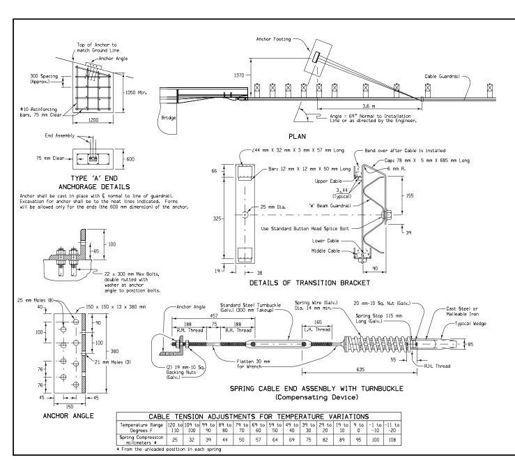
Turnbuckles shall be of the open type and shall each provide for a minimum takeup of 300 millimeters.
