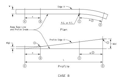
Normal Pavement Sloped in the Same Direction as Superelevation
