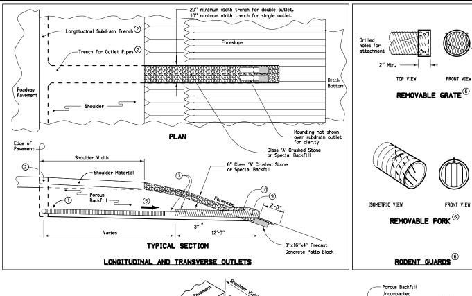
Transverse and backslope subdrains require only single outlets. Double outlet pipes shall be used on all longitudinal subdrain systems, except at the beginning and end of the system. At these locations, a single outlet nine shall be used
