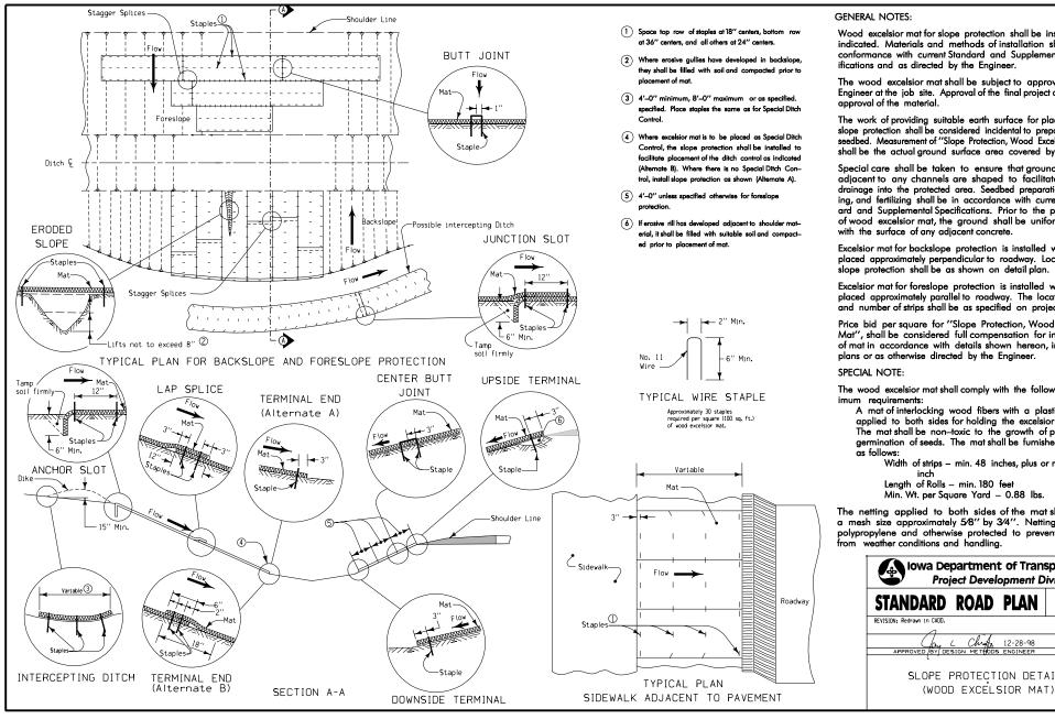
Wood excelsior mat for slope protection shall be installed as indicated. Materials and methods of installation shall be in conformance with current Standard and Supplemental Specifications and as directed by the Engineer.
