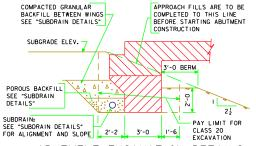
ABUTMENT EXCAVATION DETAILS SECTION NORMAL TO & ABUT. BRG.
