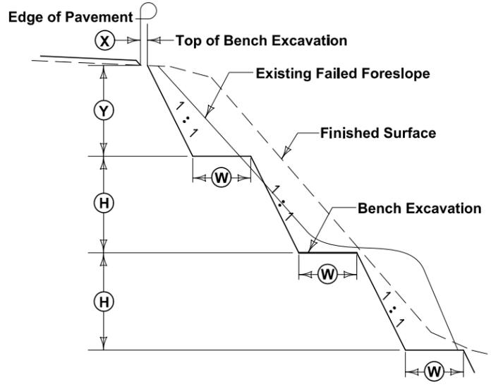
Benching height and width to be adjusted based on field conditions at the time of construction.
