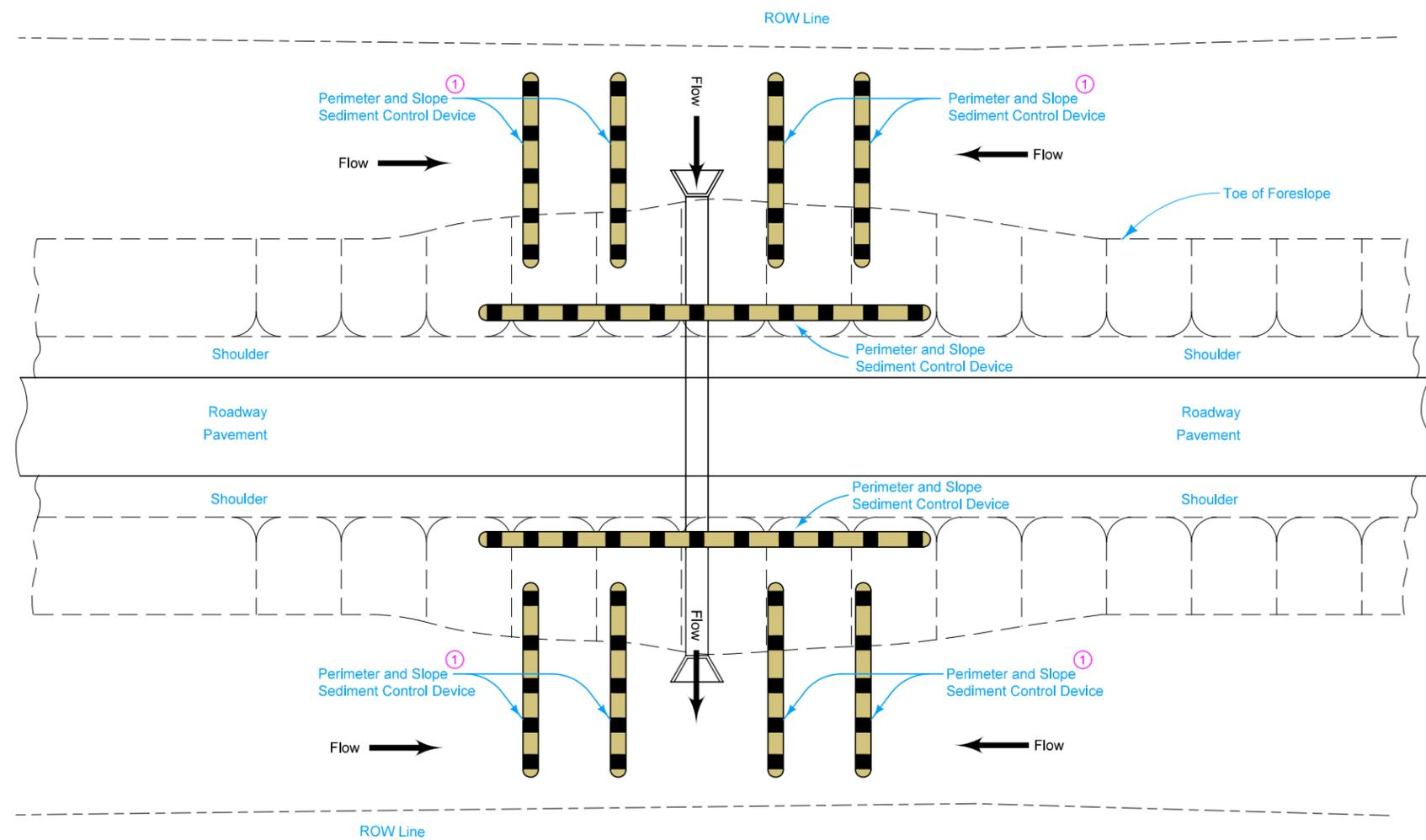
① Silt Fence for Ditch Check may be substituted at no additional cost to the Contracting Authority.
