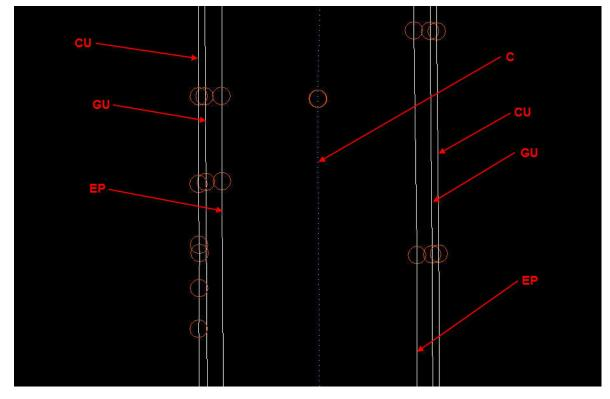
These following feature codes are used with roadways having integral curb and gutter sections.
