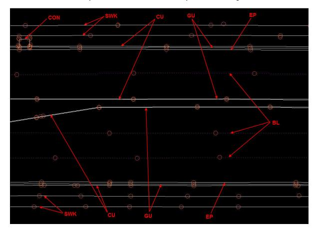
For an intersection of two roadways with curb and gutter, use these feature codes shown below.
