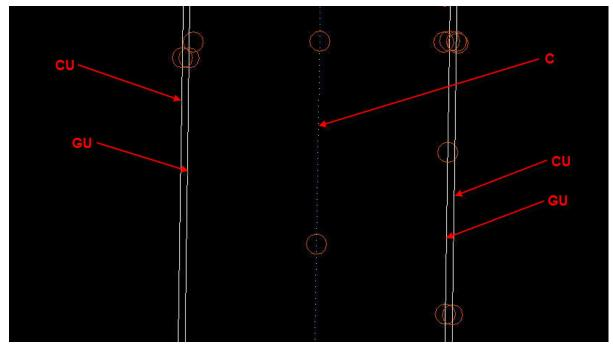
These feature codes below may be used with multi-lane roadways with curb and gutter.
