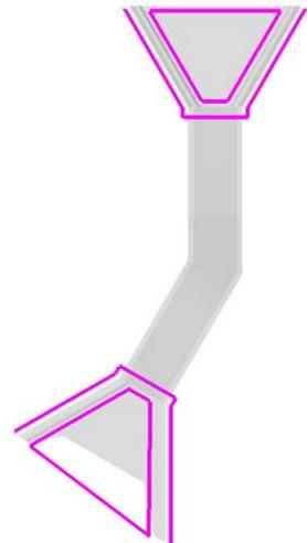
16.) The location point for the culvert is stored as an SOP feature. The location of this shot should be where the centerline of the culvert intersects the roadway alignment and at the elevation of the roadway. If the culvert does not cross the centerline, the SOP should be at the inlet flowline. The description of the SOP point should include the culvert ID, dimensions, condition, skew angle, drainage area and terrain type (F= FLAT, R = ROLLING, H= HILLY, VH= VERY HILLY).
