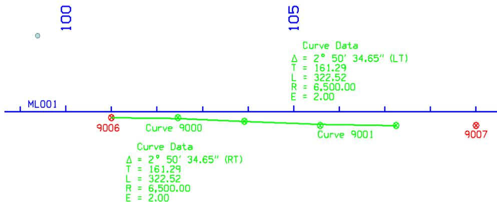
Figure 2A.6: Reverse curve for lane redirection in example problem.
