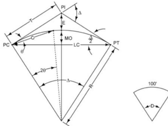
**Figure 2A.1:** Components of a simple horizontal curve.
