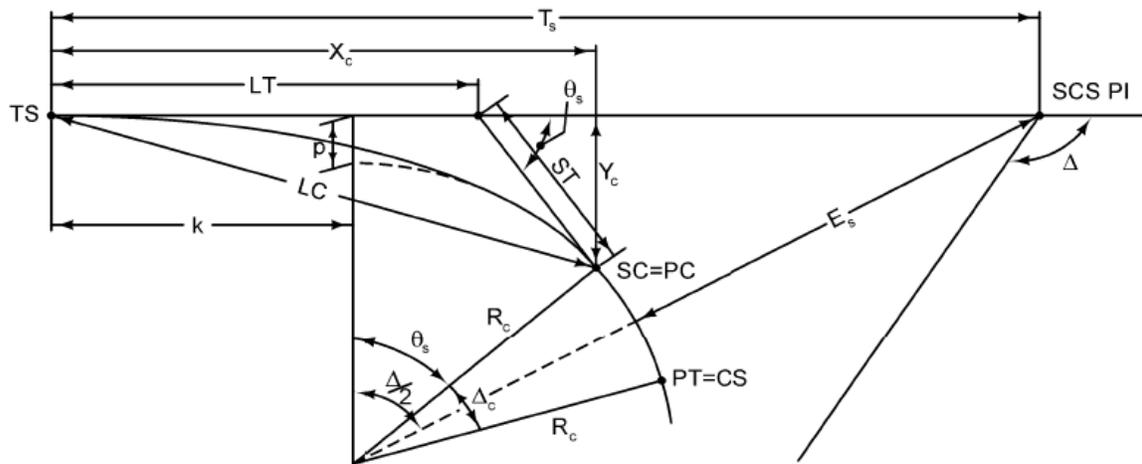
Figure 2A.8: Components of a spiral curve
