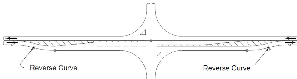
**Figure 2A.4:** Reverse curves at a channelized intersection.
