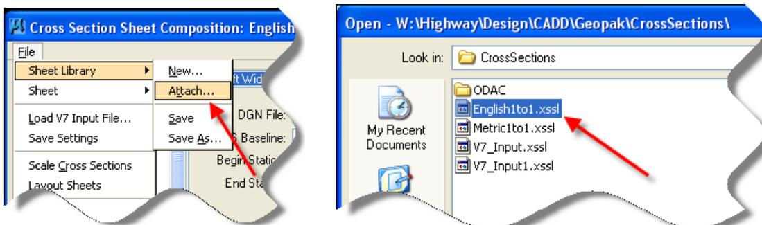
Click the drop-down arrow and from the option list select the **Active Cross-section Sheet** that is to be used to sheet the cross-sections at the desired scale, as shown at the right. (Example: 280ft Wide, Centered)
