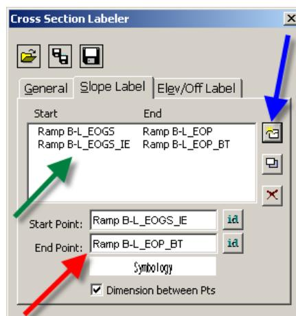
When all data input listed above is complete, switch back to the **General** tab, (red arrow at the right), and click the **Draw Labels** button, (blue arrow). This will produce the requested dimensions and slope labels, as defined in the **Attributes** dialog above, and as shown by the green arrows at the right.
