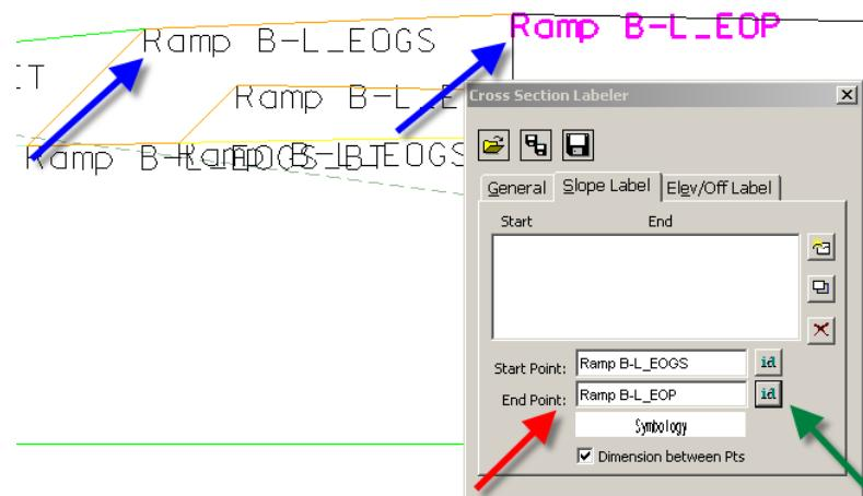
Segments to be dimensioned must be added to the list box, (as shown by the green arrow at the right.) Each pair of points defining the line segment to be dimensioned, (as shown by the red arrow at the right), must be added to the segment listing in the list-box, (green arrow), by *clicking the **Add*** button, as shown by the blue arrow.
