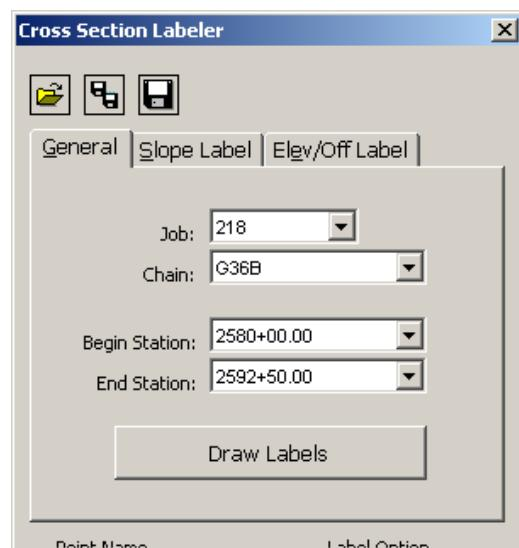
After entering the necessary **Job**, **Chain**, and **Begin and End Station** information in the data entry fields, as shown at the right, click either the **Slope Label** or **Elev/Off Label** tab.
