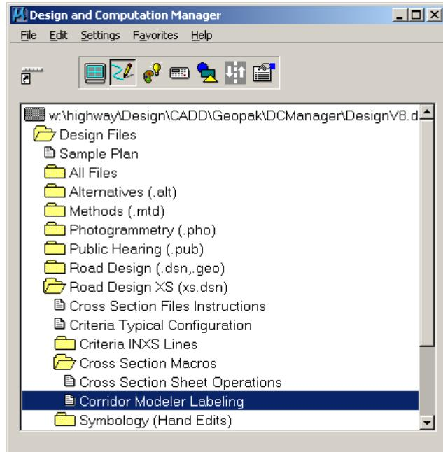
Double-clicking the **Corridor Modeler Labeling** tool, as located above, will produce the **Cross Section Labeler** dialog, similar to as shown at the right.
