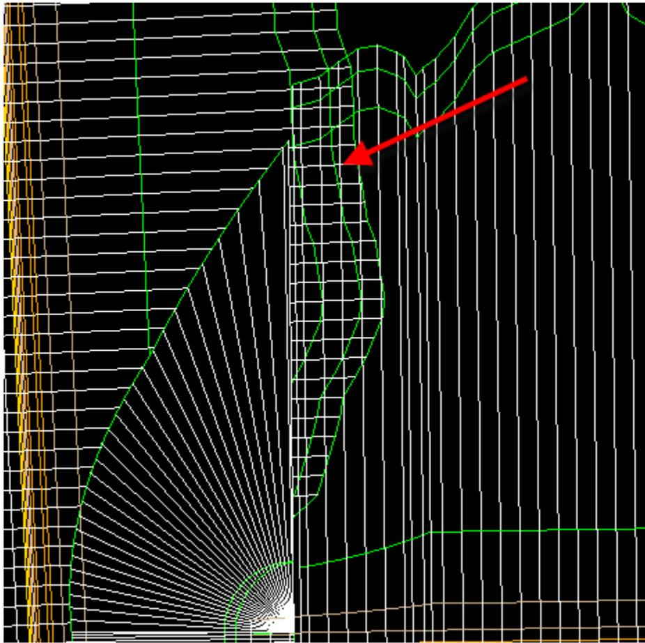
Below shows return geometry that was developed with an acute angle. Notice the breaklines for the shoulder (Orange Lines) don't quite match up. The value vs. time spent here is not beneficial.
