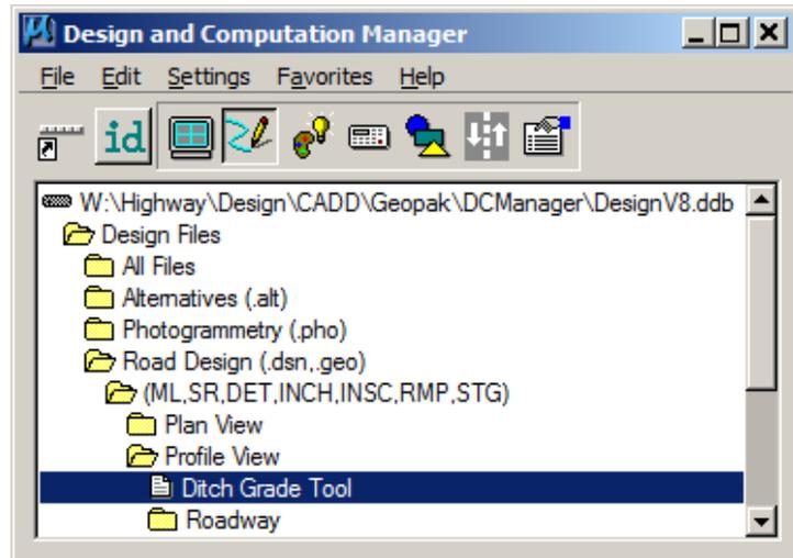
This tool is used to draw correctly formatted ditch grade information into the profile area of a model.
