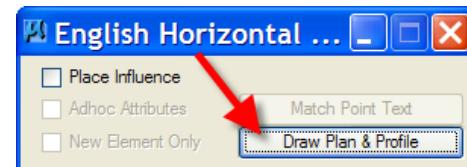
Clicking the “Draw Plan & Profile” button will activate the “Open Job” dialog, shown at the right. Select the appropriate “gpk” file, (job), and click the **OK** button. This will produce the **Draw Plan & Profile** dialog, shown below.
