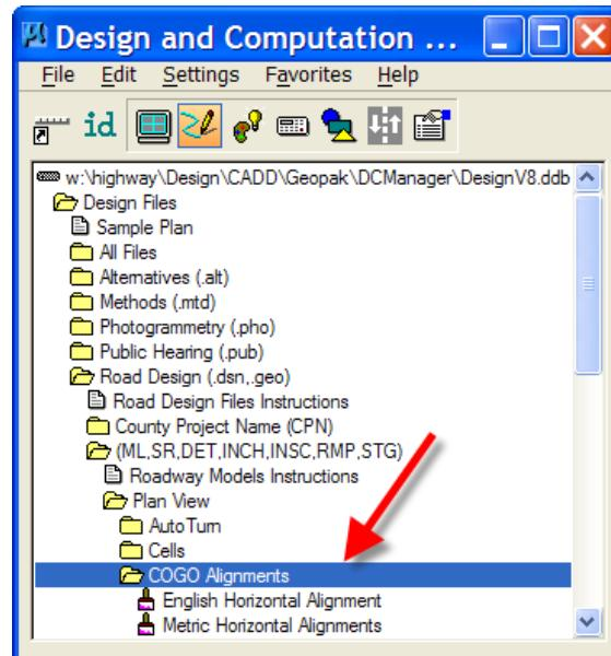
*Double-clicking* either the “English...” or the “Metric Horizontal Alignment” tool, (shown above), will run a program that will determine the resolution and scale of the open model, to be used later to populate the **Geopak Label Scale** field on the **Draw Plan & Profile** dialog.
