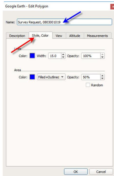
To place the polygon that will visually define the Survey Request Area, place points (left-click) to define the area, as shown to the right. The shape will not begin to display until at least three points have been placed, and will continue to change shape when additional points are placed. When the polygon shape placement is complete, click the **OK** button to accept the shape. The “**Google Earth - New Polygon**” dialog will disappear.
