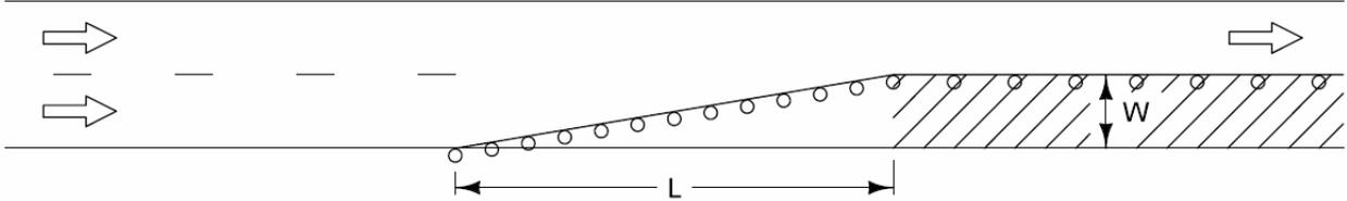
**Figure 1:** Merging taper.
