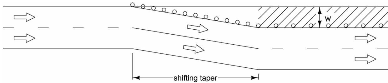
**Figure 2:** Shifting taper.
