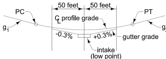
**Figure 3:** Sag vertical curve showing a minimum gutter grade.
