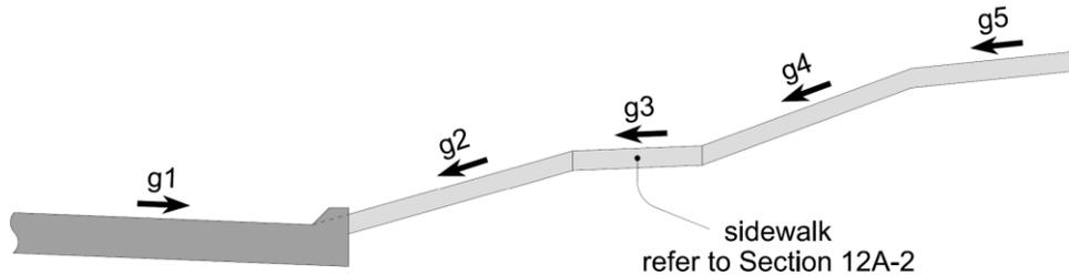
Type B, C, and D accesses: g2, g4, and g5 should not exceed 14% and should be as flat as possible for Type B high volume traffic accesses.
