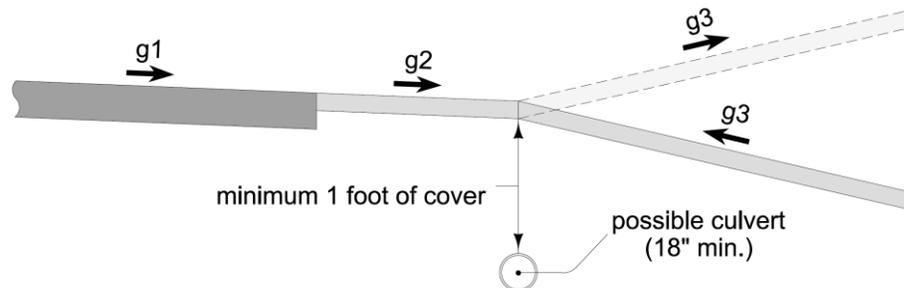
Type B, C, and D accesses: g3 should not exceed 14% and should be as flat as possible for Type B high volume traffic accesses.
