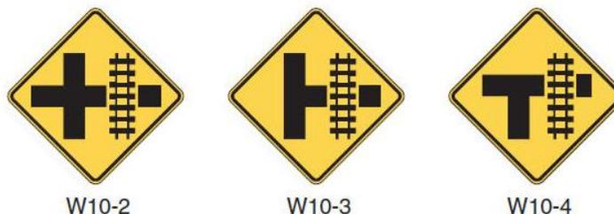
**Figure 4:** W10 series warning signs for grade crossing (2009 MUTCD).
