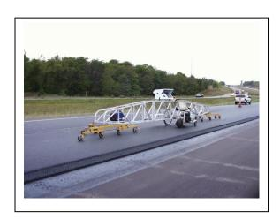
Smoothness may be measured with a 25-foot California type profilograph, which produces a profilogram (profile trace) of the surface tested, or high speed profilograph equipment, which has become the preferred choice for higher production projects.
