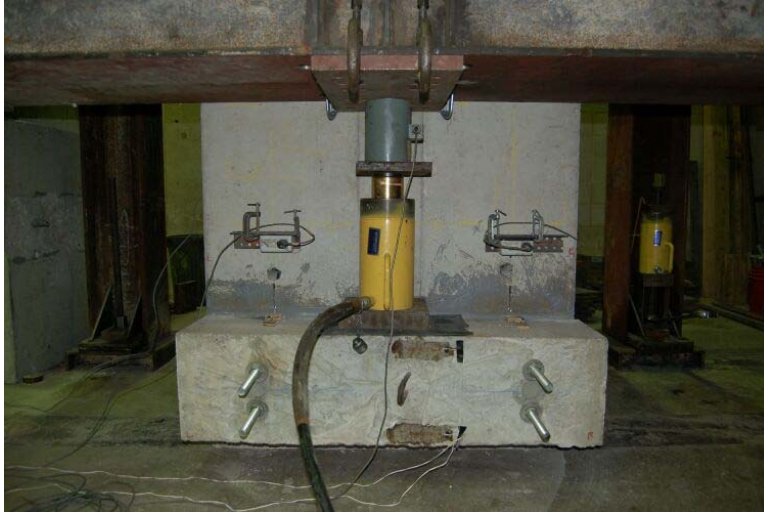
Figure 9. Ultimate load test on a specimen with four stainless rods.
