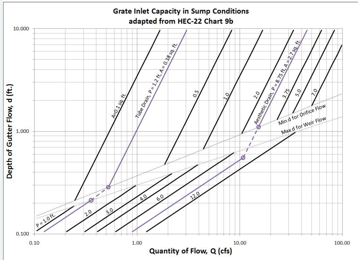
Figure 5: Grate Inlet Capacity in Sump Conditions
