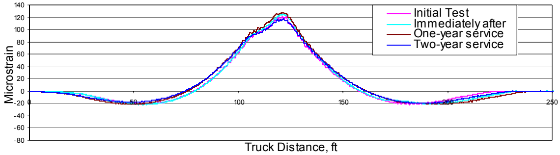
FIGURE 7. Bottom Flange Strain Data (Path Y2, Beam 1 on Center Span of Bridge 1)
